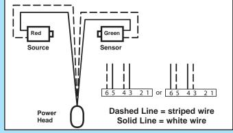
FIG. 4-5a Source and sensor wiring methods.
